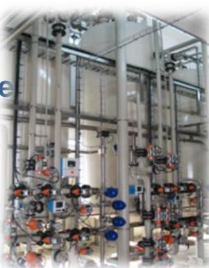
Industrial references, development of high temperature (65°C) EDBM technology (lower footprint -25%), better control of bacteriological development, processing of viscous products)
